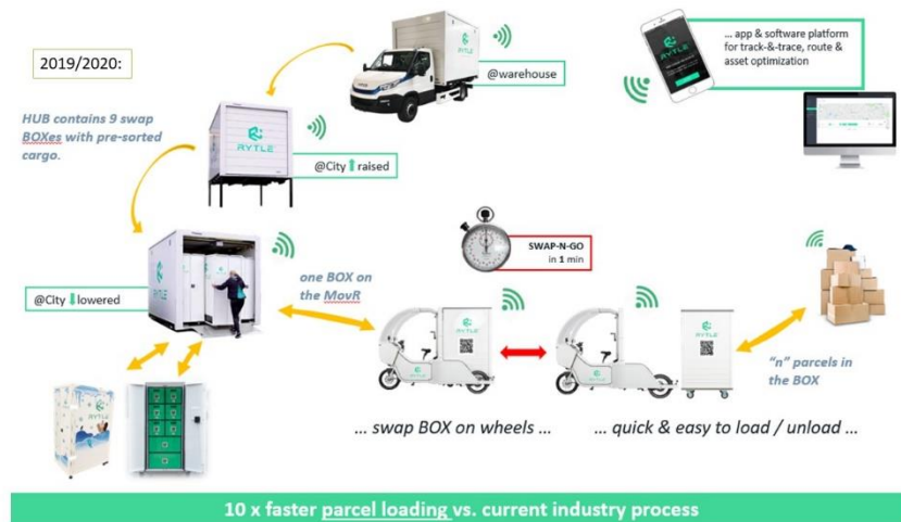
Figure 14 Rytle technical solution – infographic
