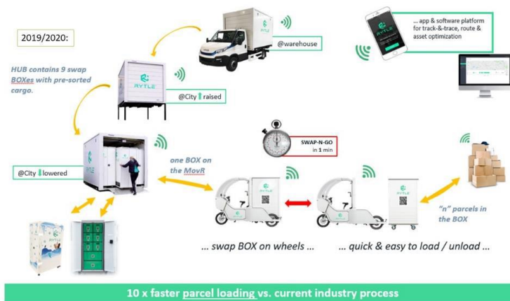
Figure 5: Technical solution promoted by Rytle for the shared public microhubs in Bremen
